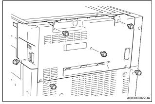
3. Remove the right upper cover from the machine (two screws).
