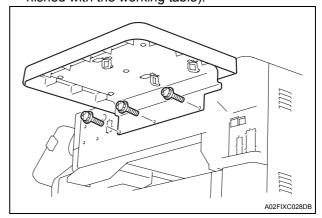
6. Install the mounting bracket (two places) (two screws A each furnished with the working table.)
