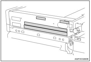
9. Secure the working table (three screw B's furnished with the working table).
