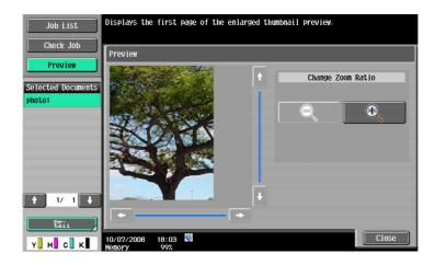
Enlarge the image of the document to check details. The image can be magnified 2 times, 4 times or 8 times. To view the desired portion of the enlarged image, use the scroll bars located in the right and the bottom of the image.
