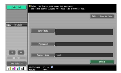
Enter the account name and password, and then press either [Login] in the touch panel or the Access key on the control panel.
