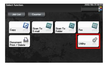
[Utility] allows you to configure settings of this machine, register destinations, and check the status of consumables.
