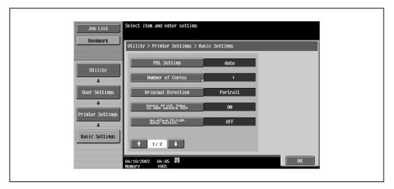
4 Press the [C] (clear) key to erase the value, and then use the keypad to type in the number of copies. (1 - 999)
