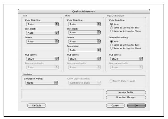
When printing, color processing is performed according to the selected ICC profiles.
