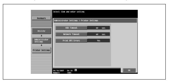
3 Press the [C] (clear) key to erase the value, and then use the keypad to type in the time. (10 - 1,000 seconds)
