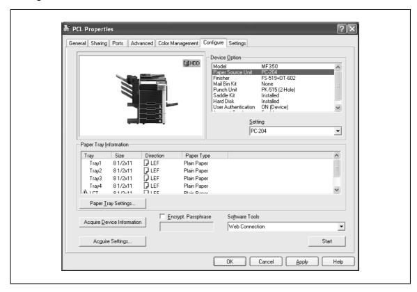
The functions of this machine can be used from the printer driver if the model name used, installed options, the User Authentication and Account Track functions are specified.
