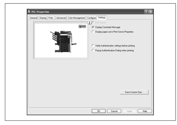
The default settings for displaying the confirmation messages or the dialog box for entering the authentication settings can be changed.
