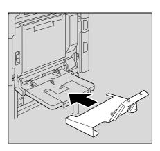
6 Erect the guide of the mounting kit.
